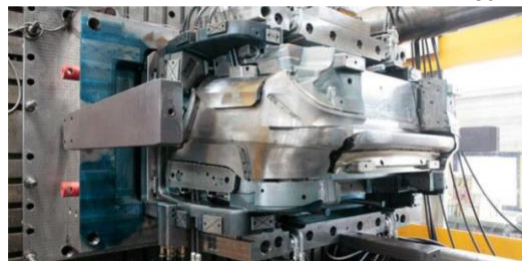
Figure 3: Half of an injection mould for a front bumper Source: Schneider Form GmbH
